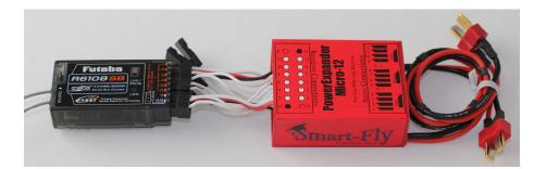
PowerExpander Micro-12G connected to a Futaba R6108SB 8-channel receiver
